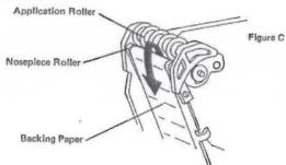
1. Remove cover from left side of tool by pulling out at top.
