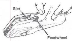
Squeeze operating lever several times until backing paper exits labeler. If backing paper does not become taut and exit at rear, remove backing paper from slot and repeat steps 6 and 7.
