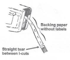
Completely squeeze operating lever, exposing feedwheel. Insert backing paper into slot. When paper bows up, maintain finger pressure and release operating lever.
